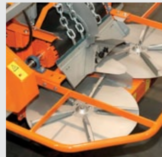
Wet lime spreading unit
